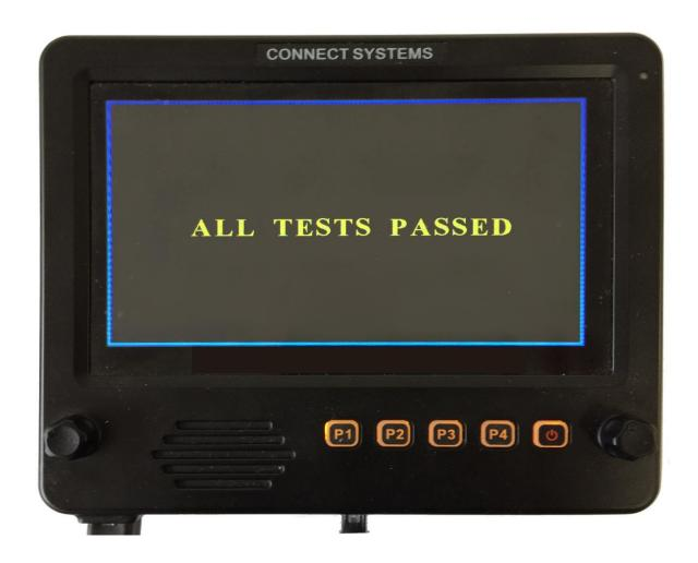
In order to have all test passed, it is necessary to make shorting plugs for USB1, USB2, and the UART port.
