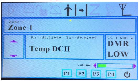
Notice the screen name is "Temp" and the other parameters is what was programmed in the previous screen. You are ready to press the PTT button on the microphone and start talking to someone.
