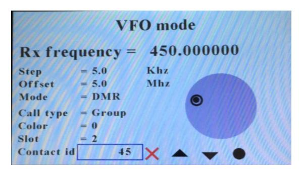
To change the parameters, use the up and down arrow to select the parameter as shown above.
