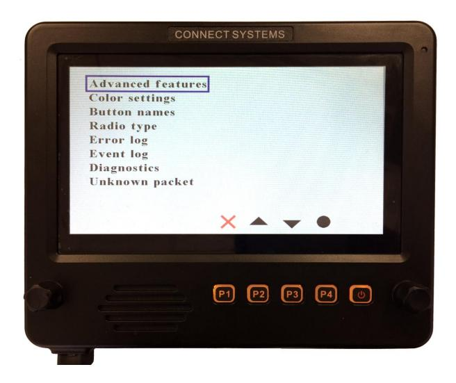
The up and down arrow on the touch screen or P2 or P3 will select which feature you want to select. The solid circle on the touch screen or P4 will select that feature that is highlighted. To exit from this menu select press the Red X on the touch screen or P1.
