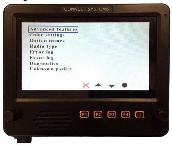
The up and down arrow on the touch screen or P2 or P3 or the right rotary switch will select which feature you want to select. The solid circle on the touch screen or P4 will select that feature that is highlighted.
