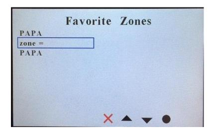
After you finished entering the zone number, press the "O" key from the keypad of the DTMF microphone, the P4 key, or the black circle on the display above the P4 key.
