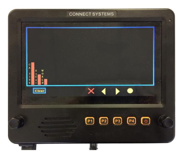
If you let the CS-BFD monitor a repeater for a length of time, the CS-BFD will gather the activity on the channel and display it in graphical form as shown in the above screen. If you want to see the details of the various groups, press the right arrow key or P3 and you will get the display shown on the next page.
