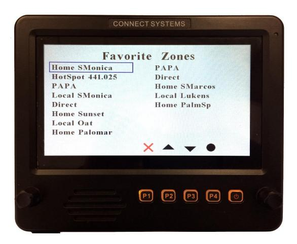
To select a favorite zone, use the right rotary knob or the up and down keys to select the zone you want to jump to and then press the solid circle or the P4 key. Alternatively, press the favorite zone on the screen.
