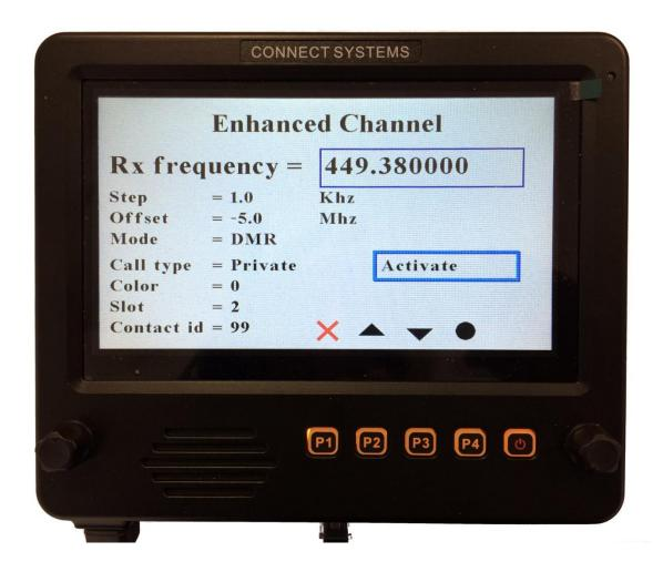
To move between parameters in this and other menus, the box around the parameter must be blue. When it is red it means you can change the value of the parameter. The change the active parameter position, use the right encoder, the up and down arrow keys, or P2 and P3.
