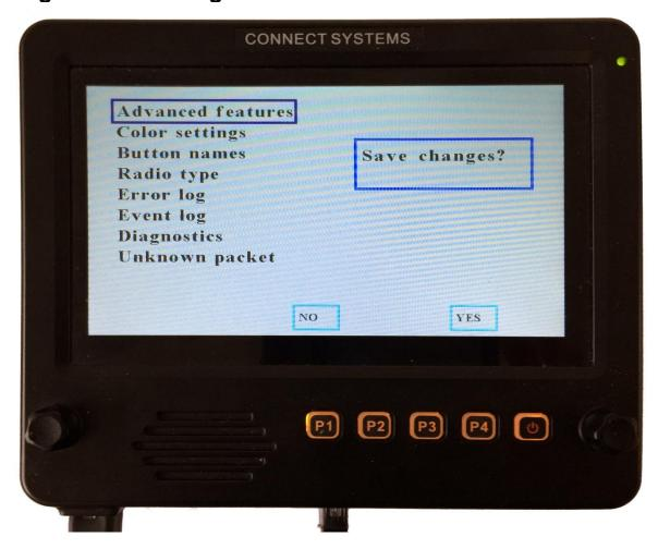
Press the Yes or P4 key and you are finished. Pressing the rotary switch on the right will return you to the main screen as shown below.
