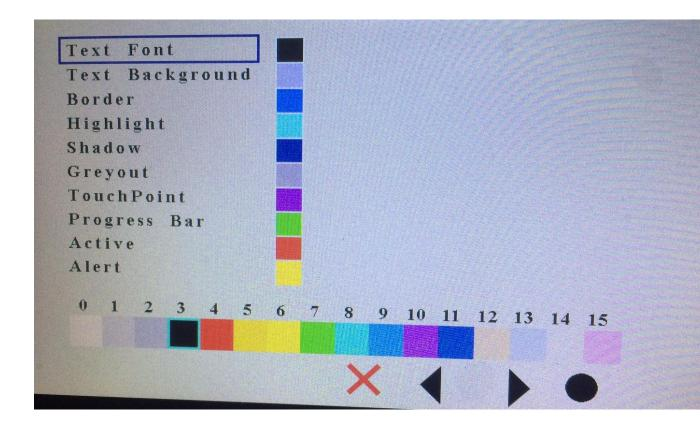
Use the left or right arrow key or P3 or P4 to select the color you want and then press the Select key or P4 to lock it in. around the key and the color of the selected item has changed to that color as shown below.
