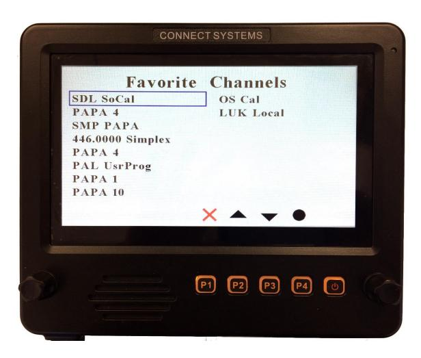
To select a favorite channel, use the right rotary knob or the up and down keys to select the zone you want to jump to and then press the solid circle or the P4 key. Alternatively, press the favorite channel on the screen. If you want to add a new favorite channel, first move the box to a free channel or to an existing channel.
