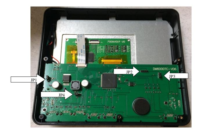
JP1 is used to determine the source of its power. If the jumper is between the center pin and the pin closest to the top of the display, then the power is derived from the radio. If the jumper is between the center pin and the bottom of the display, then the power is derived from an external power supply.
