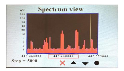
You can select between the step sizes by the right encoder or the up and down keys on the display, P2 and P3, and the keypad on the DTMF microphone. Once you select the size press the select key.
