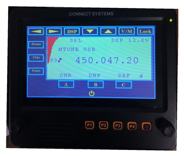
There is one unusual feature available due to the limitation of available knobs. P1 is used to select normal operation of the radio where the knob on the right is used like the channel selector on the original display and the knob on the left is used for the select knob like on the original display.
