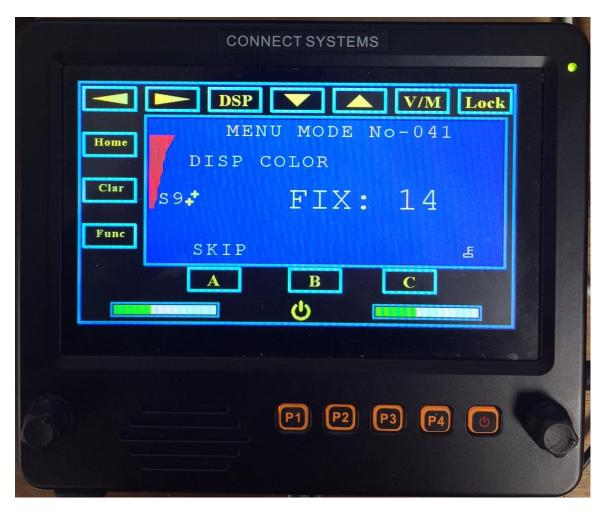
The knob on the right is used for the volume control and the knob on the left is used for squelch control. Once you set levels the way you want them, press the P1 switch again to get out of that mode. Menu Mode # 41 from the FT857D allows you to set the color. The following screens shows some of the colors available:
