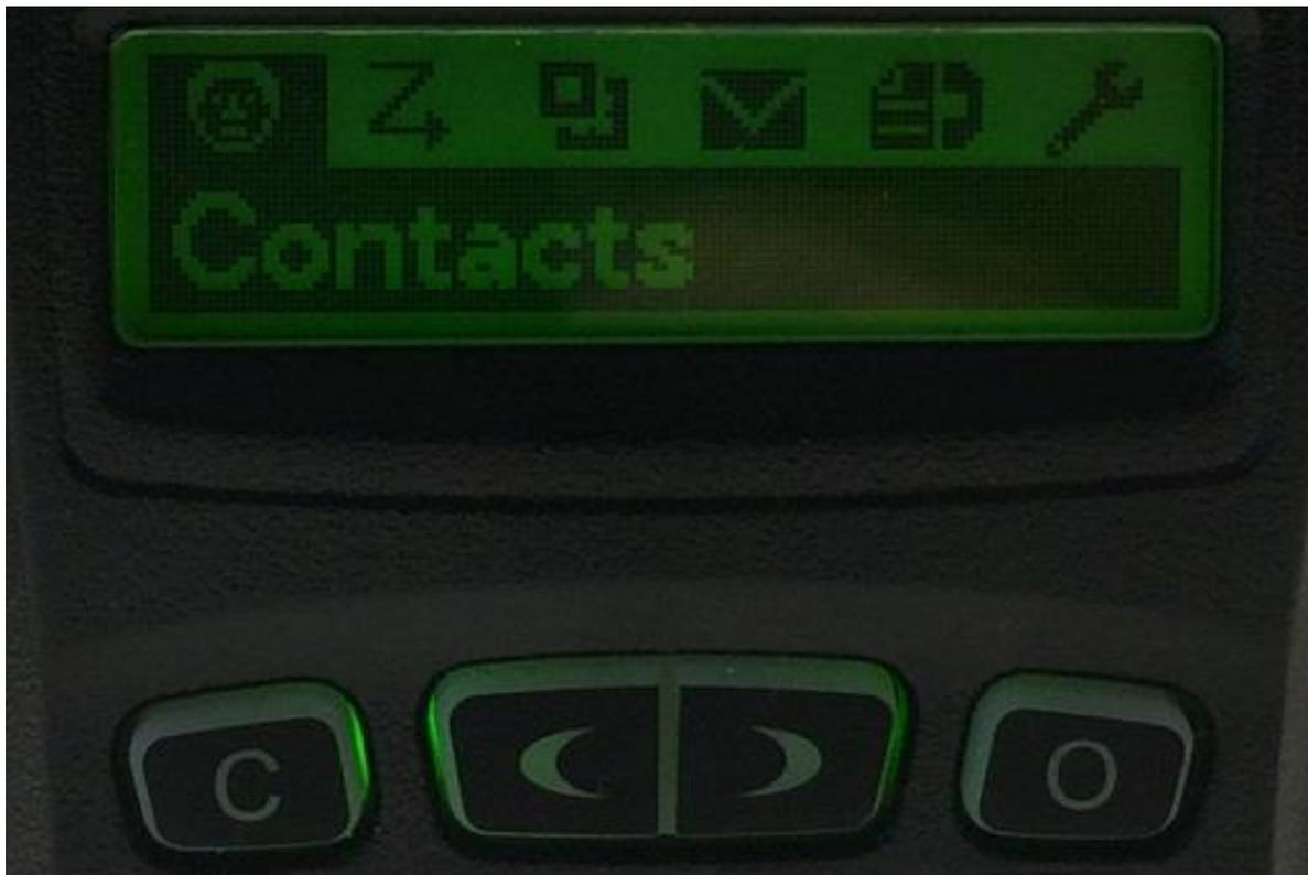
Press “)” key multiple times to scroll right or “(“ key one time to scroll left and you get the following screen:
