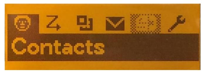
Press P3 multiple times to scroll right or P2 one time to scroll left and you get the following screen:
