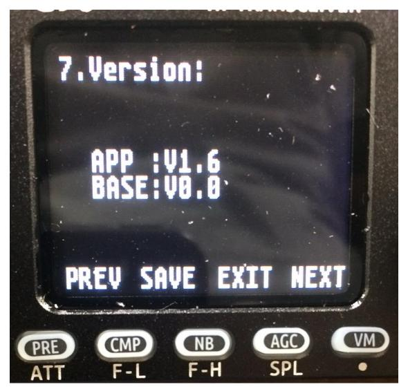
This screen above is an example of where the firmware was not loaded correctly in both the main unit and the display. In this case the base was loaded with version 1.7 and the display had version 1.6. The screen below shows where the firmware has been updated correctly. Note that the version that has been loaded is version 1.71.
